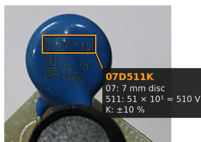
VR1: 07D511K varistor 7 mm, 510 V, across L-N (DERIVED 0.90)
